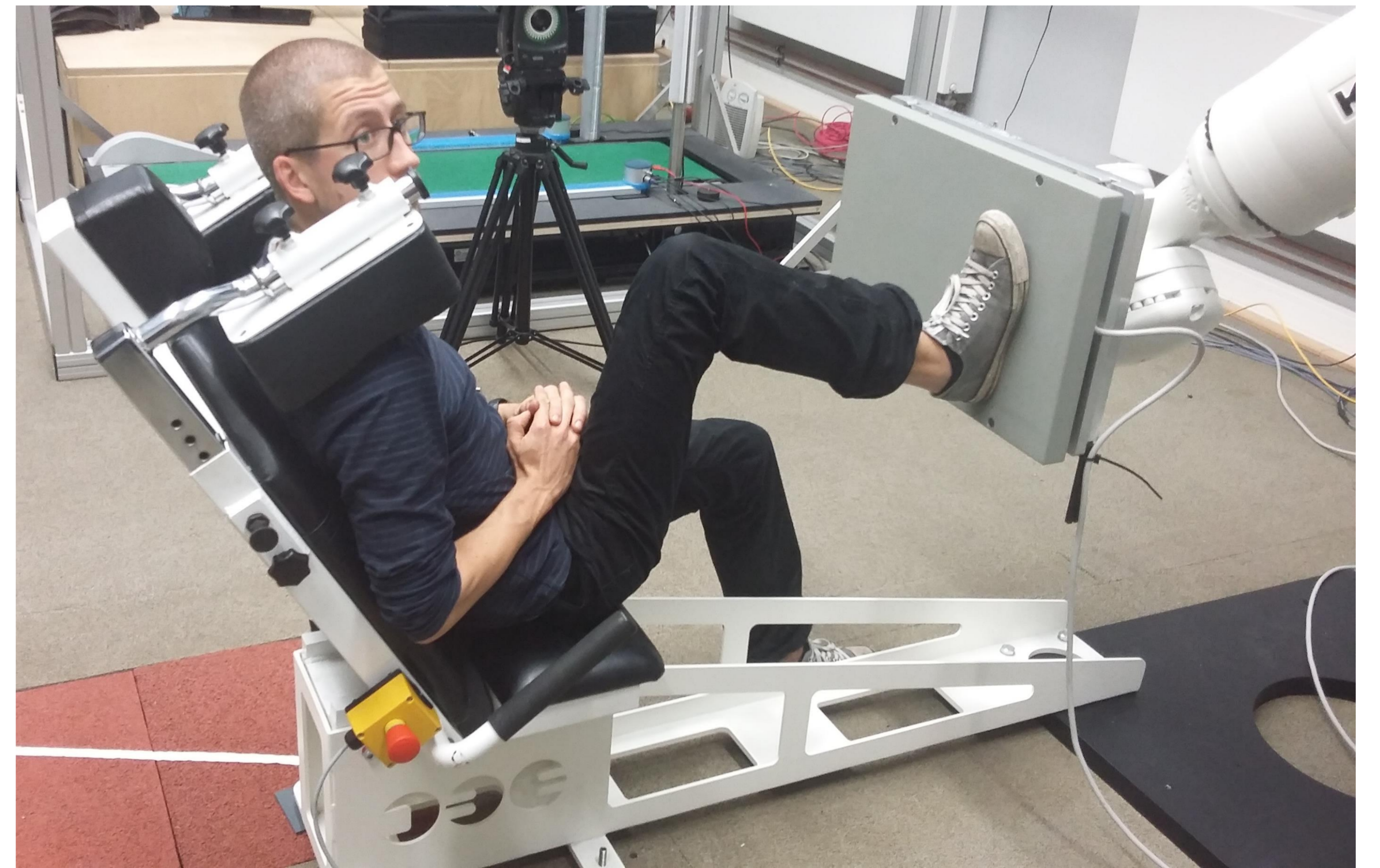
Fig. 3: Visualization of the novel robotic leg press training device. The actuator (KUKA KR 270 R2700 ultra) of the training device should be able to control the resistive force, movement velocity and range of motion by applying individual training trajectories.
