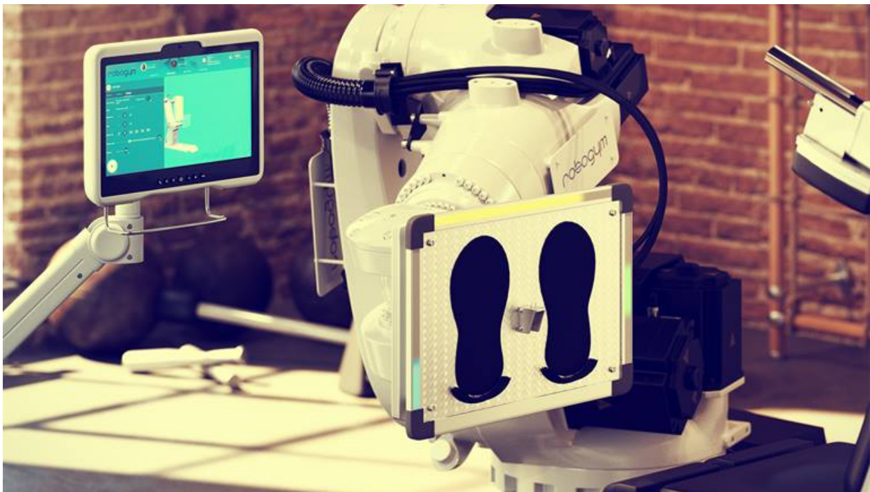
Leg press with sensors for force measurement and a screen with training data
